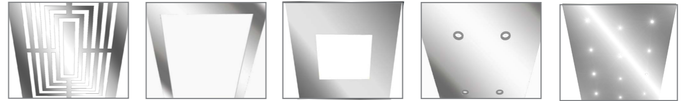
Labyrinth patterned drop-down ceiling | Plexiglass lighting | LED panel lighting | Spotlight lighting | Starry sky (LED point lights)
